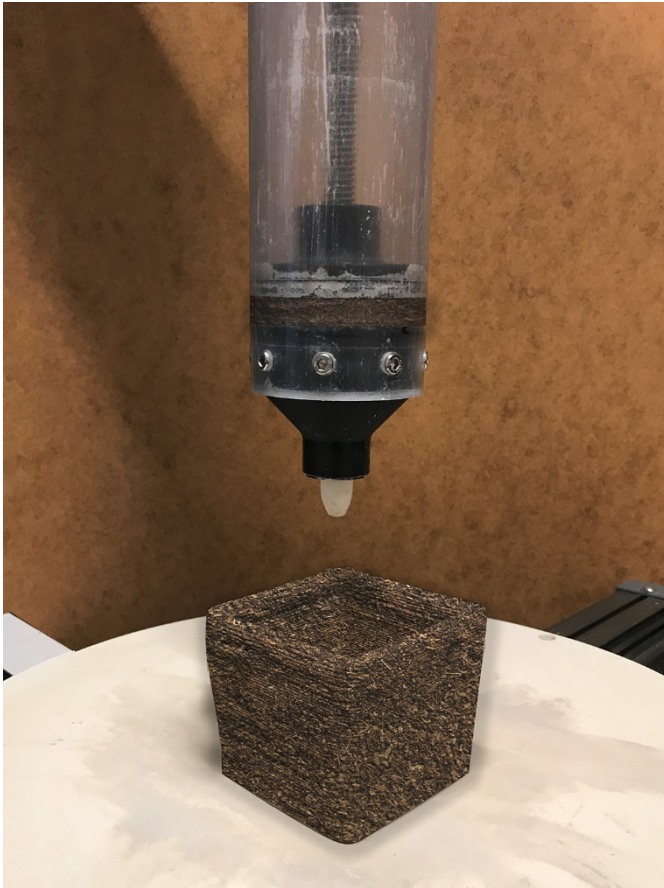
Picture 1: 3D printing of a sample based on mycelium.
